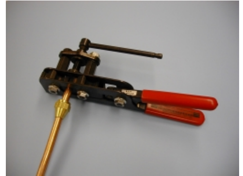
2 Use a flaring tool or punch to flare the tube end at 45°.
