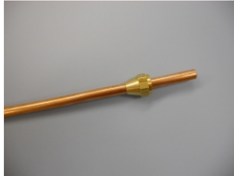
1 Slide the flare nut over the copper tubing used to attach the impeder.
