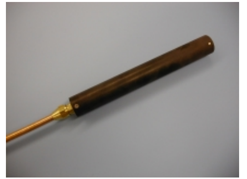
4 Thread nut onto impeder to provide leak tight coolant connection.
