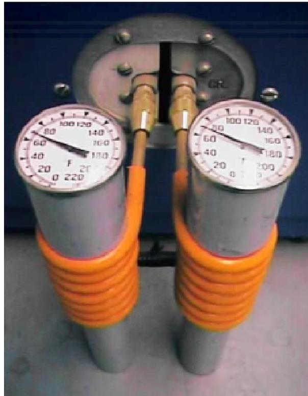
Each sample is placed in a simple calorimeter, with a measured amount of water sufficient to cover the samples. Each calorimeter is then placed within two identical inductors which are
