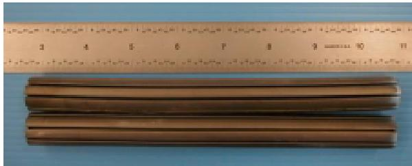
The photograph above shows ferrite that has excessive bow. This is a common problem that requires additional clearance be allowed between the ferrite & the inside of the impeder tube. The bow reduces the mass of ferrite that can be used in a given size impeder, & thus degrades performance.
